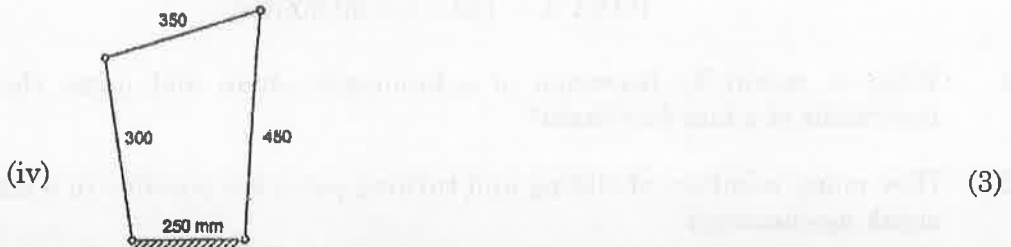
Fig. 11 (a) Four-bar mechanism All dimensions are in 'mm'
